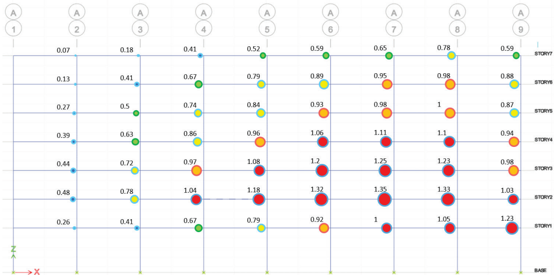
Figure C-26 AR Beam Negative Moment, ASCE 41: BSE-2N - Soil Compression only (CP)
