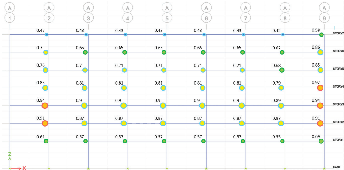
Figure C-24 ARs Beam Negative Moment, ASCE 41: BSE-2N, - Fixed Base (CP)
