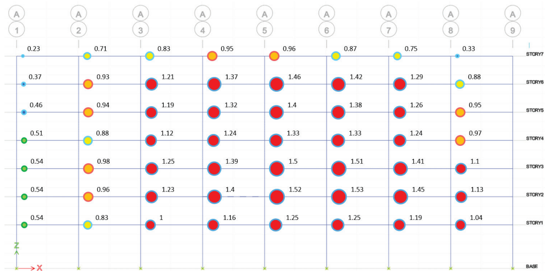
Figure C-30 ARs Beam Positive Moment, ASCE 41: BSE-2N - Compression only (CP)
