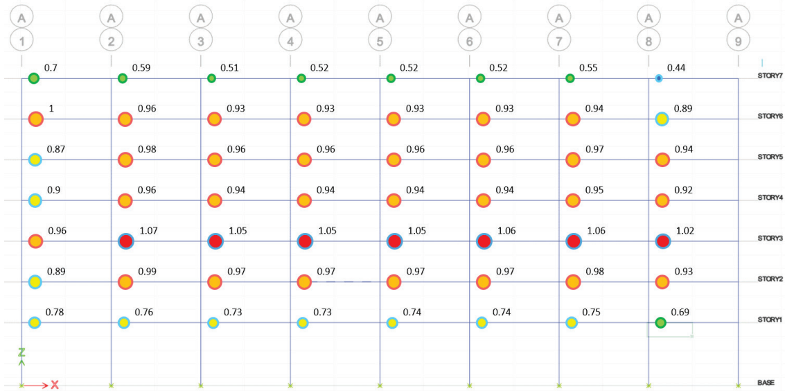
Figure C-29 ARs Beam Positive Moment, ASCE 41: BSE-2N - Soil Takes Tension (CP)
