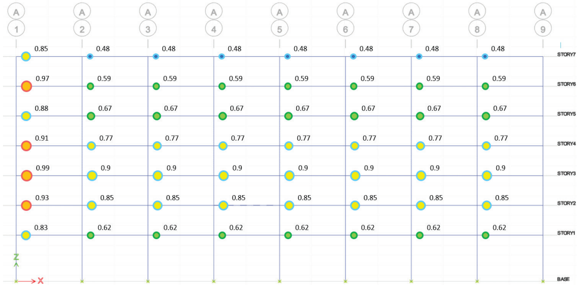
Figure C-27 ARs Beam Positive Moment ASCE 7: BSE-1N - Baseline
